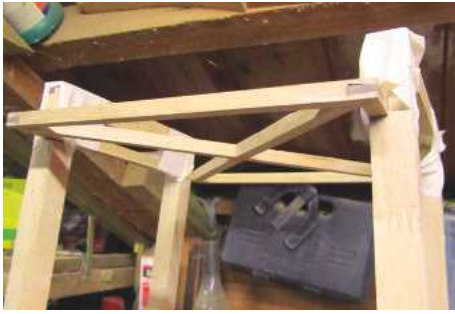
▲ Pic 1. Trying to work out the appropriate size for intermediate shelves – given the splay on the legs – made Tony’s head hurt. It was simpler to make the top and bottom shelves first, then hold the structure together with masking tape
